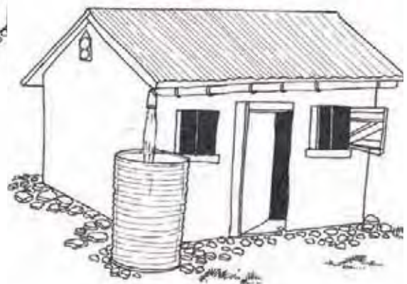
Figure 7: Domestic roof water harvesting that frees up labour and time for other economic activities
