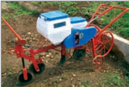
PLATE 26: Chisel-type fertilizer boot (furrow opener) behind cutting disc; offset double-disc seed furrow opener at rear. Brazilian type animal traction no-till planter, used in various countries.
