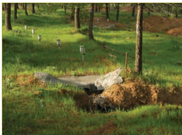
Figure 27: Measuring rainfall and the resulting surface runoff generated by the forest surface; Yatir forest; Israel.
