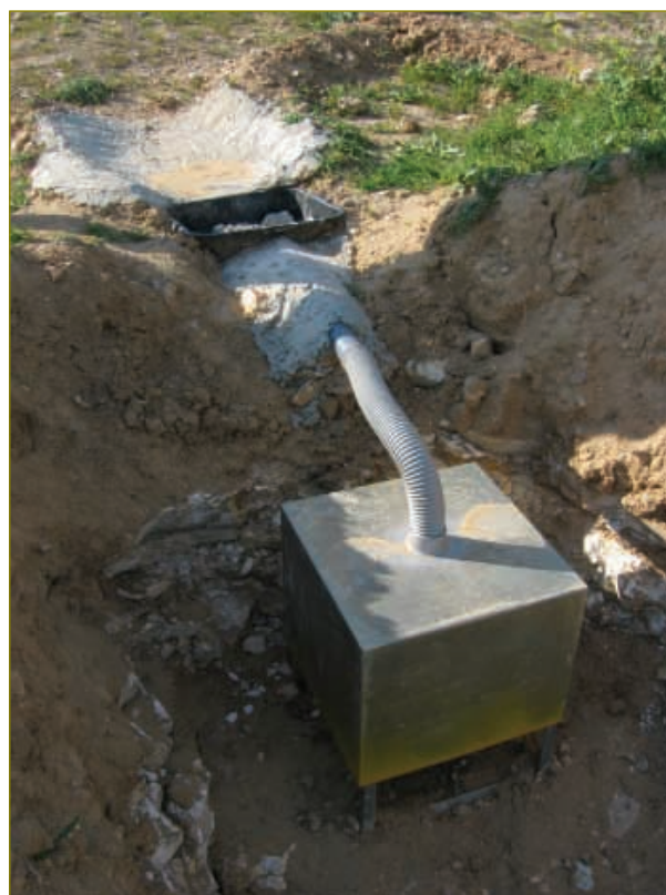
Figure 28: Water collection and measurement through tipping buckets (inside box); Israel.
