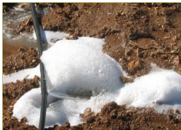
Figure 72: (Primary) Treated Wastewater. Visual appearance gives first indication of water quality and often causes social rejection of wastewater reuse, especially on food crops.
