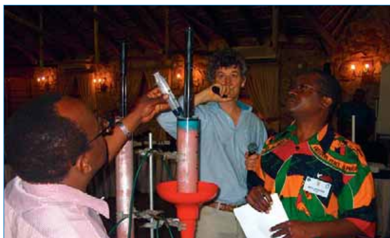
Figure 2. The wetting front detector is an ideal tool to help farmers and advisors gain a better understanding of water and solute movement. Sponges representing the topsoil, subsoil and soil below the root zone are 'irrigated' to show the movement of the wetting front (above left). A sand filled Perspex tube, irrigated with different coloured water, is used to show how irrigation affects the movement of salt and fertilizer in the soil profile (above right).
