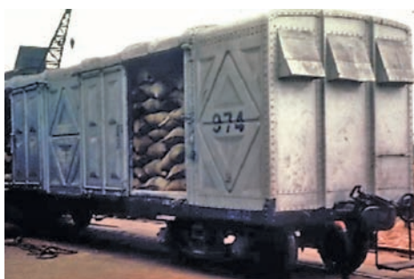
FIGURE 17 Freight containers can be fumigated if they can be made gas tight. Sealing end ventilators on this container will be difficult
