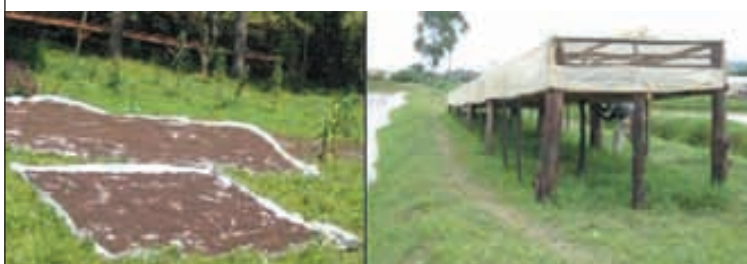
FIGURE 16 Sun drying fish pellets (left) and (right) wind tunnel feed dryer
