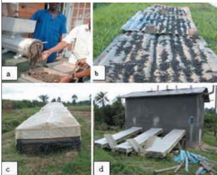
FIGURE 5 Feed processing and drying (a) feed pelletier (b) direct sun drying on corrugated iron sheet (c) solar dryer (d) improved solar dryer
