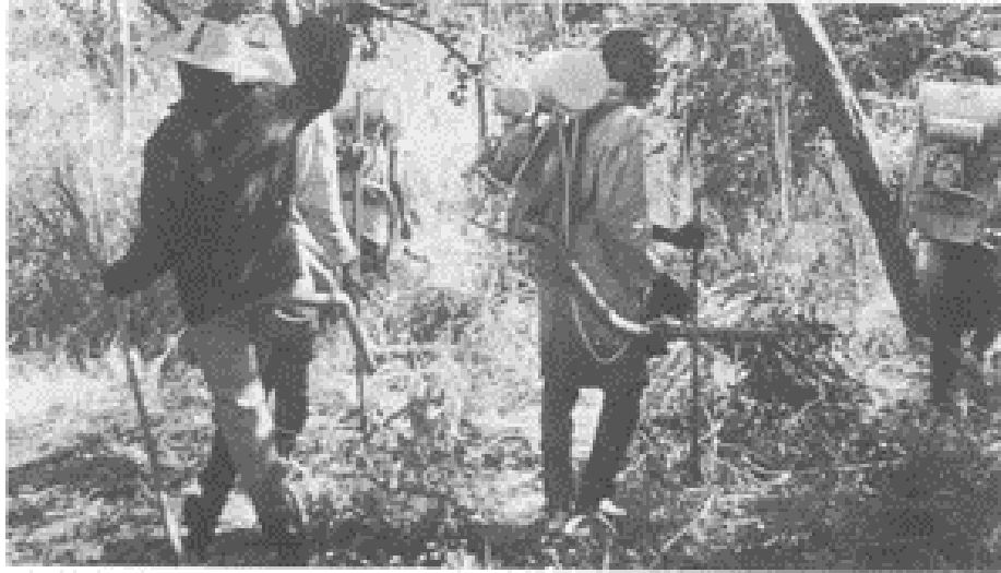
Above Motorized knapsack mistblowers in use against infestation in dense habitats
