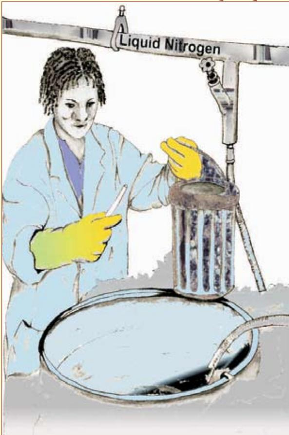
*Collecting liquid nitrogen from a big container to a small flask*
