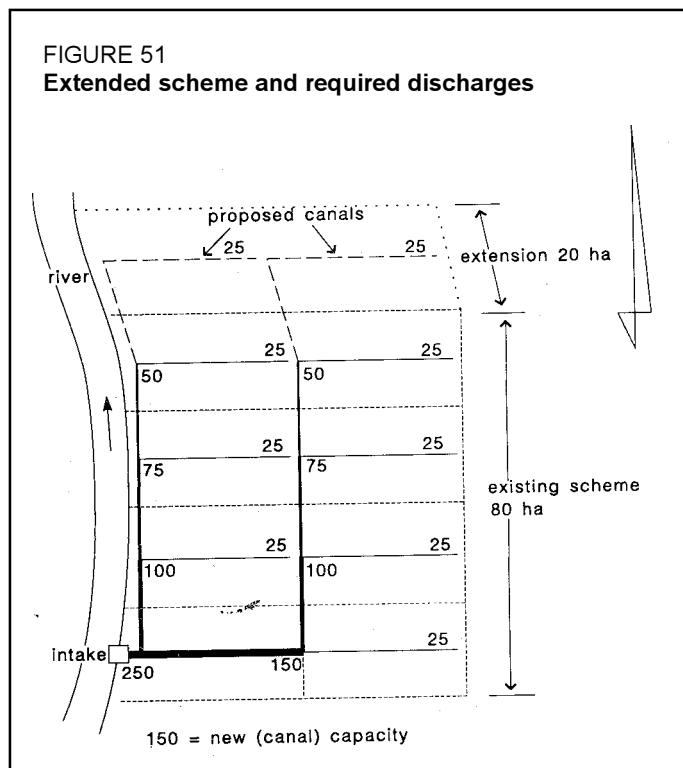
**Step 7** If necessary, enlarge the capacities of the existing canals
