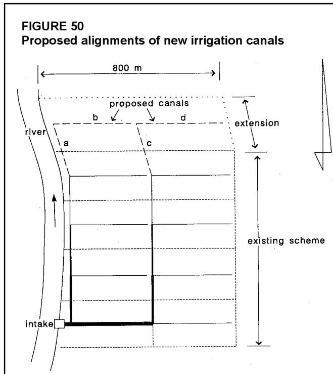
**Step 5** Add the irrigation water needs of the extension area to the needs of the existing scheme, and check the capacity of the water intake structure and of water availability
