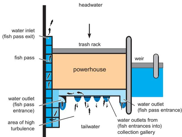
**Fig. 3.10:** Diagram of an American hydroelectric power station with a collection gallery (after LARINIER, 1992d)
