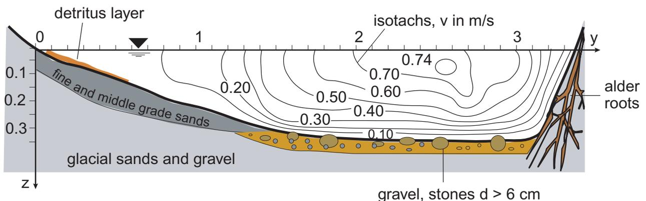
**Fig. 2.4:** Substrate distribution depending on flow velocity
