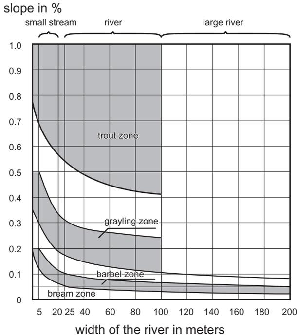
**Fig. 2.10** Graphical representation of the relations between slope, river width and river zoning for determination of indicator fish zones (modified from HUET, 1959). The typical core zones are shown in grey; the zones lying between the grey fields are transitional zones. However, these transitions take place gradually in rivers.
