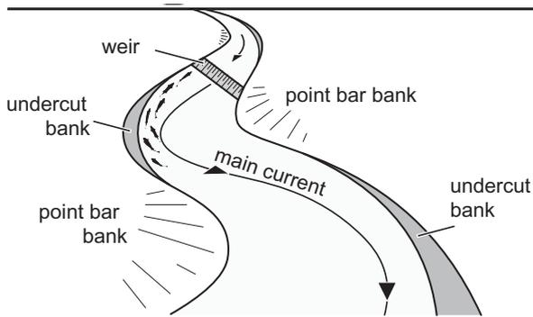
**Fig. 3.4:** Diagram showing the flow pattern in a river with undercut banks and point bar banks. Fish swimming in or along the main current will arrive at the weir along the side of the undercut bank. Consequently, a fish pass should be positioned as closely as possible to the point where the fish meet the obstacle (modified after JENS, 1982).
