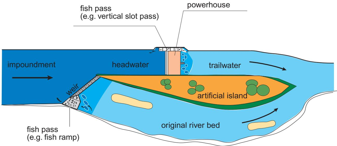
**Figure 3.7:** Ensuring longitudinal connectivity at a bypass hydroelectric power station through construction of two fish passes, i.e. one directly at the hydropower plant and the other at the weir.
