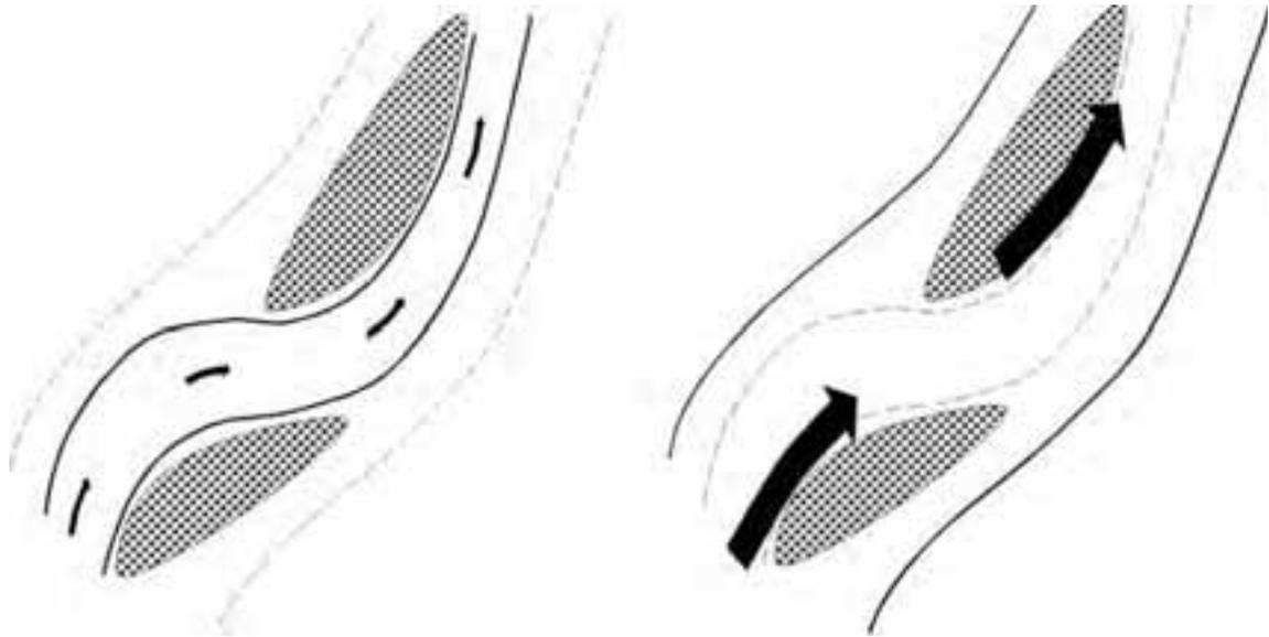
**Fig.2.3:** Changes in flow characteristics in a river at different discharge conditions
