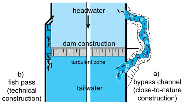
**Fig. 3.5:** a) Optimum position of a bypass channel and
