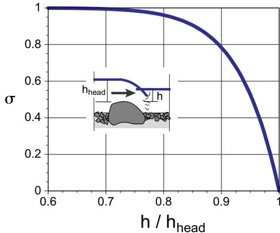
**Figure 4.46:** Drowned-flow reduction factor  $\sigma$
