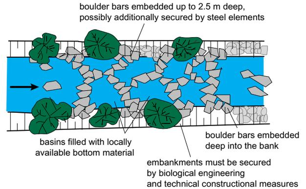
**Fig. 4.5:** Bottom step in boulder bar construction (plan view)
