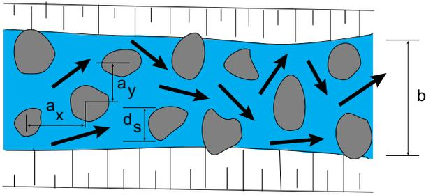
**Fig 4.19:** A bypass channel in which perturbation boulders have been placed
