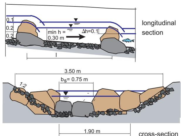
Fig. 4.48: Sketch to illustrate the example of calculation
