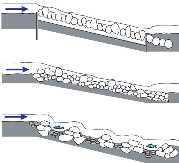
**a) Embedded-boulder construction (dressed construction):**
