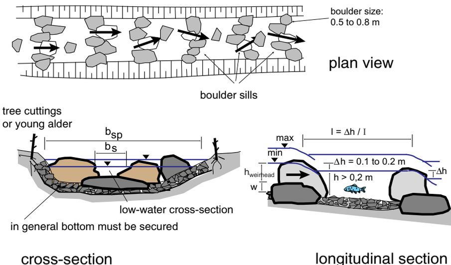
**Fig 4.20:** Boulder sills for breaking the slope in a bypass channel
