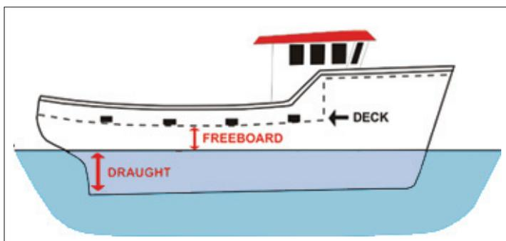
Draught relates to the depth of water required for a vessel to float freely and is measured vertically from the underneath side of the keel to the waterline.
