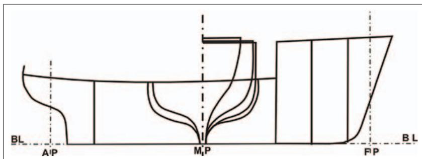
When the shape of the hull of a vessel is known, the designer, often a naval architect, can calculate the centre of buoyancy (**B**) for the various combinations of displacement, trim and heel.
