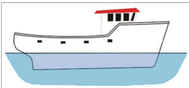
For a vessel to float freely in water, the weight of the vessel must be equal to the weight of the volume of water it displaces.
