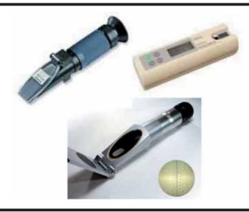
Figure VII.1.6. Refractometer for TSS measurement
