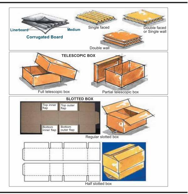
Figure VII.3.4. Nature of corrugated fibreboard, telescopic and slotted boxes
