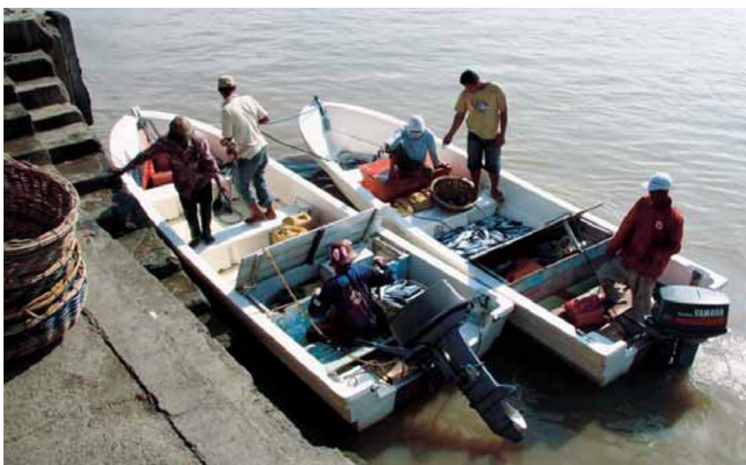
Outboard propelled glass fibre boats in Pelabuhan Perikanan Pantai (PPP) Banda Aceh port used for transport of catch from larger fishing vessels offshore. This method of bringing in catch from nearby fishing vessels is used particularly when the catch is too small for it to be economically viable for the fishing vessels to go to port and land
