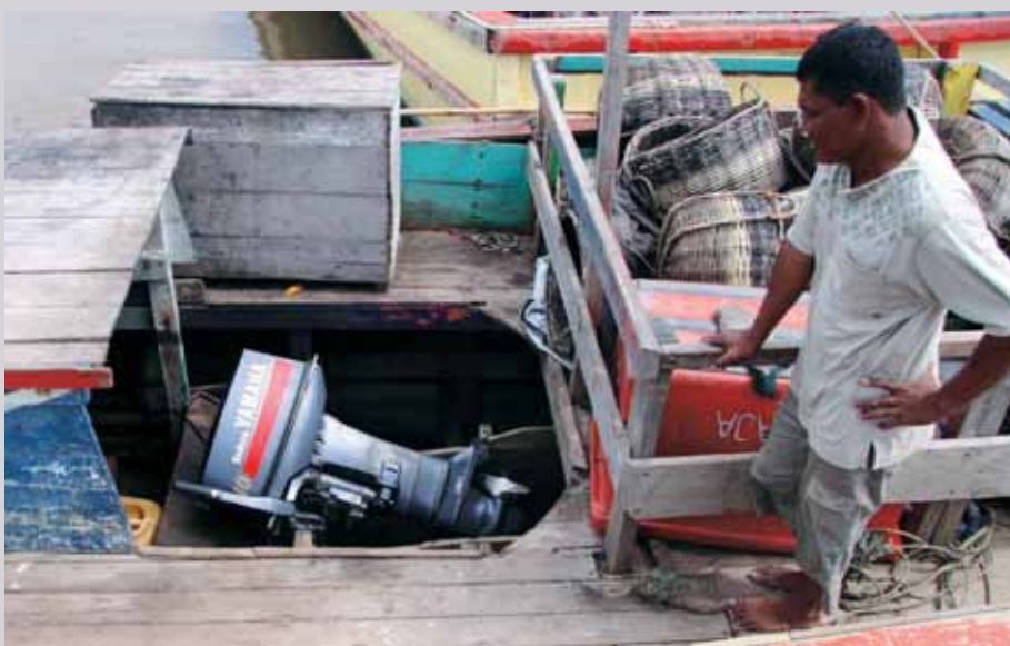
The 40 Hp outboard engine that is used to propel the fishing vessels
