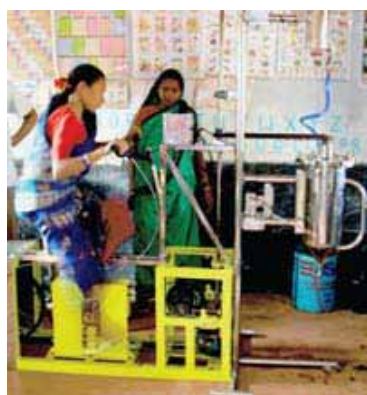
Pedal-driven biodiesel reactor (Photo: CTxGreEn)
