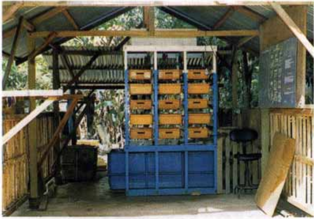
Plate 23 : A small-scale depuration unit.
