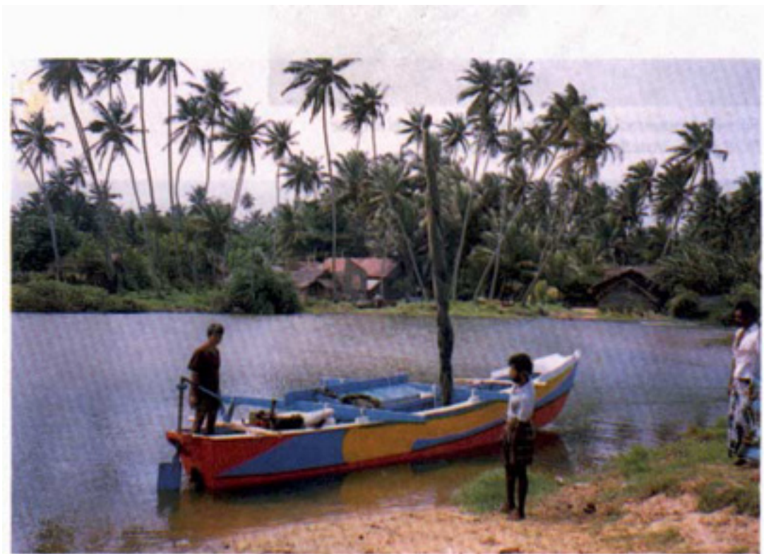
8.5 m timber outrigger canoe, SRL-18A, fitted with top mounted Yanmar air-cooled diesel engine BOB Drive
