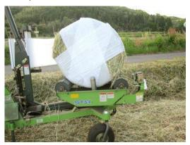
Roll-bales are wrapped tightly in plastic film by wrapping machine
