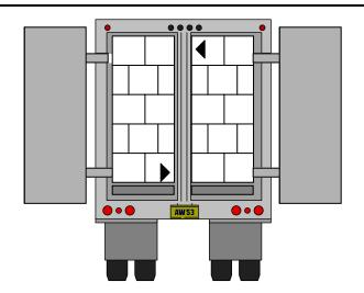
Sampling positions for a loaded vehicle
