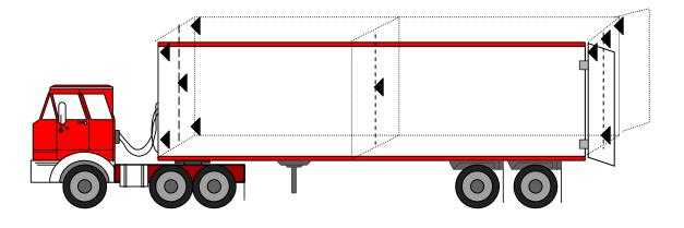
Sampling positions for an unloaded vehicle
