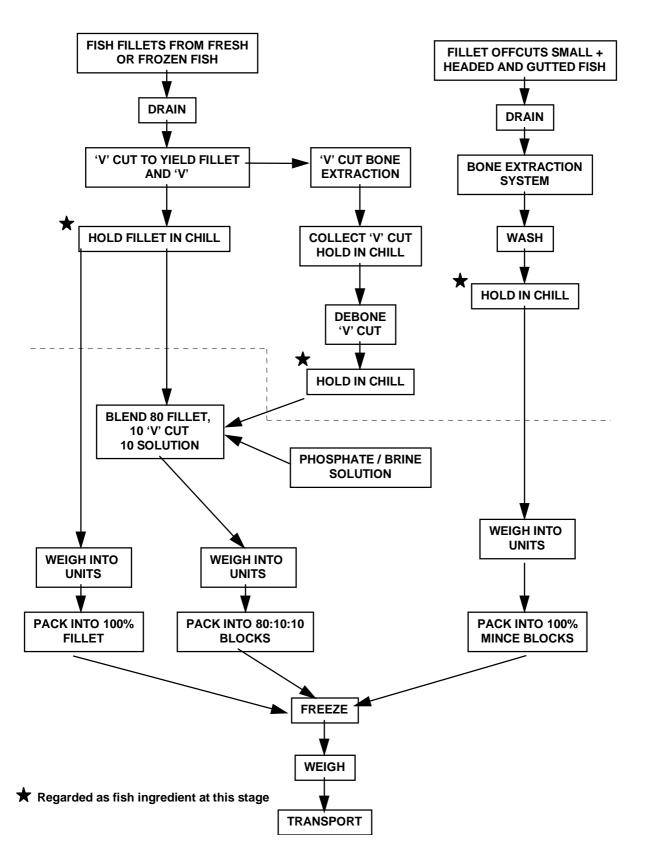
**TYPICAL PROCESS FOR FISH BLOCK MANUFACTURE**
