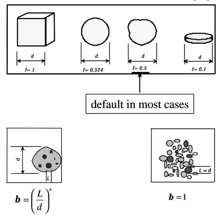
The particle shape factor f, (upper part) and liberation factor  $\boldsymbol{b}$  for un-liberated material (lower left) and liberated material (lower right). L is the liberation size of the critical particles.
