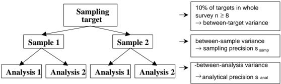
Balanced experimental design for empirical estimation of uncertainty (i.e. Two-stage nested design), using the 'Duplicate method'.
