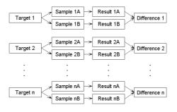
Design of experiment to estimate the bias between two sampling methods A and B, by collecting paired samples at each target.
