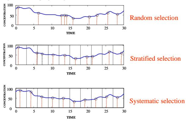
Ten samples selected from the target by using *random*, *stratified* random and *systematic* stratified sample selection.
