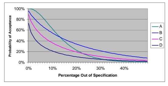
Curves C and D are the OC curves (in the presence of measurement error) for the more stringent plans appearing in the same section of the table in CGS, namely AQL = 2.5% (n = 11, k = 1.51) and AQL 0,.65% (n = 8, k = 1.96) respectively.
