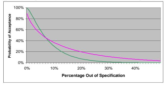
This graph shows an increase in both producer's and consumer's risks caused by the measurement error. Obviously a decision would have to be made whether these increases in risks were acceptable, but such decisions would have to be made on a case by case basis, considering the variation of the product and the measurement errors in each application of the sampling plan. This approach does not seem to lend itself to use in generic standards.
