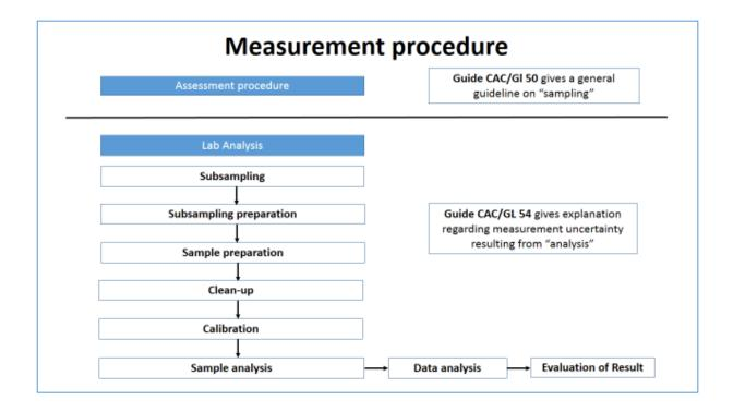
Figure 1: General steps for measurement procedure
