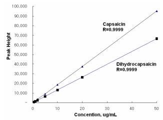
Fig. 1. Calibration curve of capsaicin and DHC by HPLC method.
