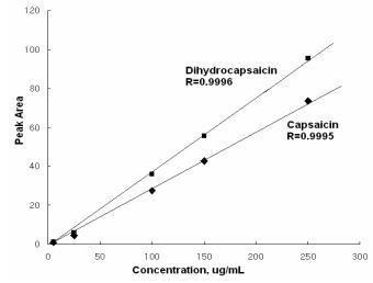
Fig.1. Calibration curve of capsaicin and DHC by GC method.
