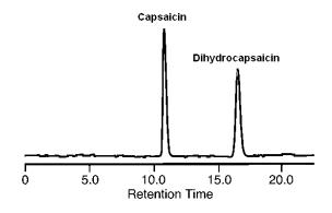
Fig. 2. HPLC chromatogram of standard capsaicin.
