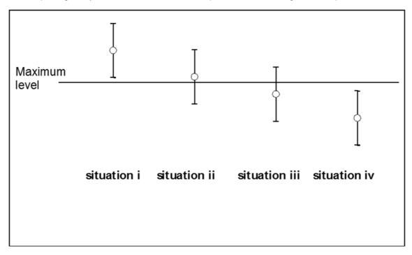
*Figure 5:* Comparing test results with a Maximum Level taking into account the expanded measurement uncertainty
