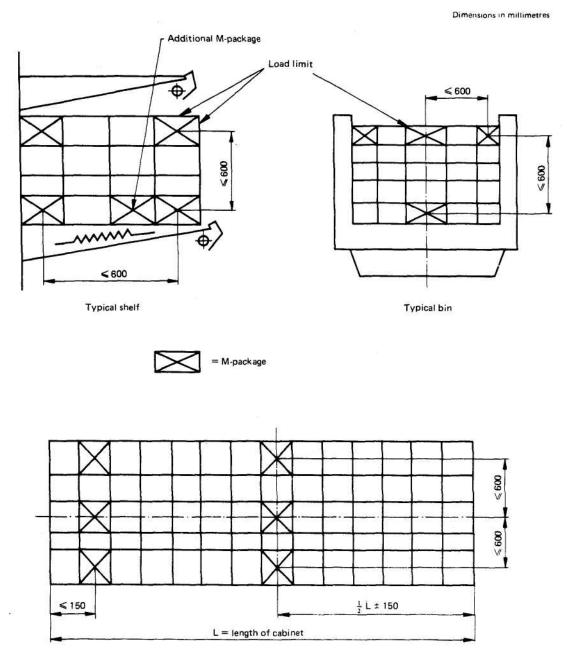
FIGURE 1 Location of M-packages (test packages with temperature sensor)
