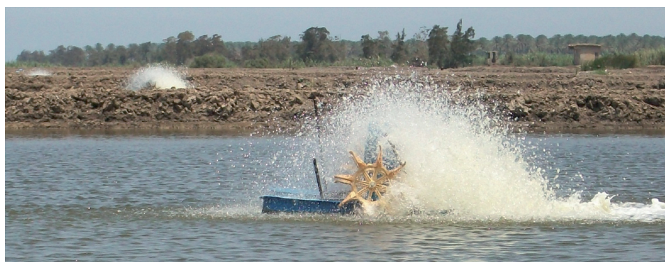
FIGURE 9 Intensive tilapia pond in Barsiq fish farm, Behaira, Egypt being aerated with paddle wheels
