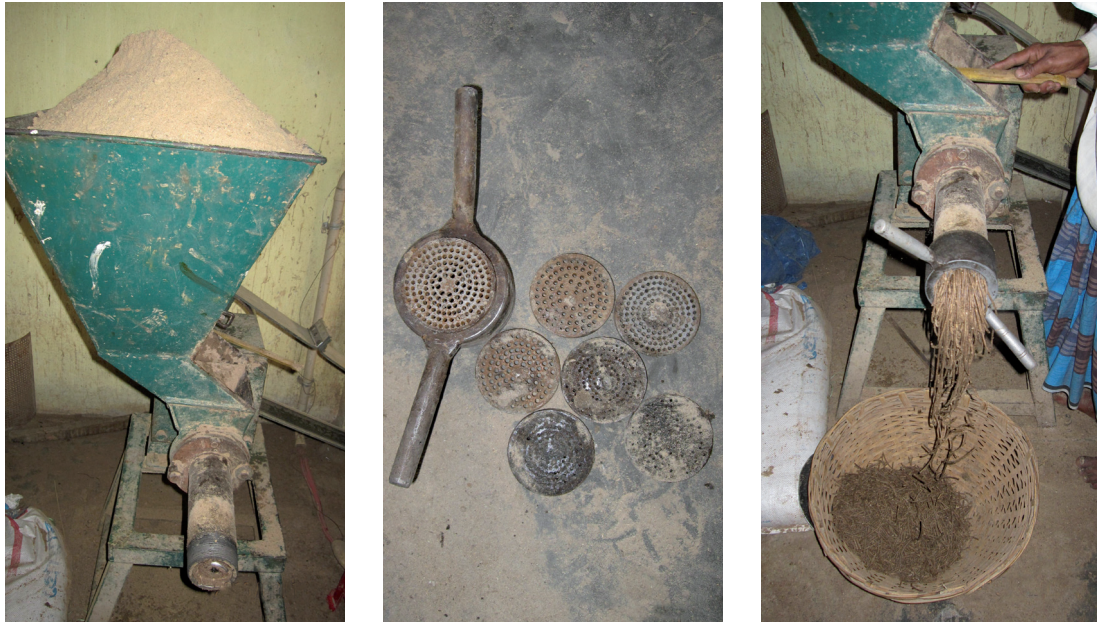
FIGURE 13 Mixed feed ingredients placed in the pellet machine (left), pellet dyes of different sizes (middle) and pellet production (right)
