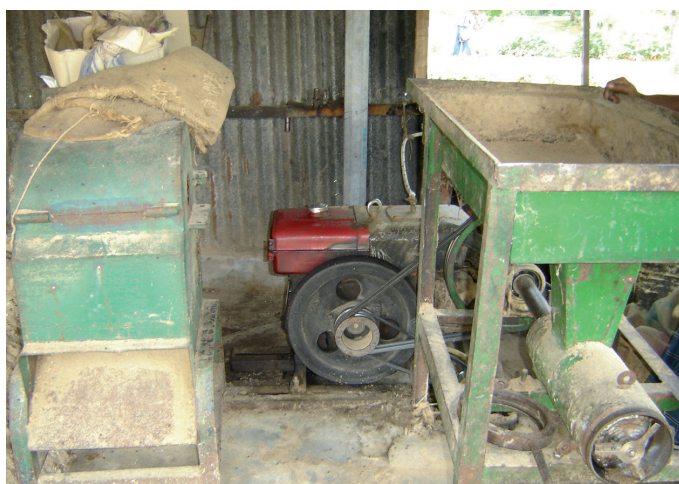
FIGURE 7 A machine for preparing farm-made aquafeeds
