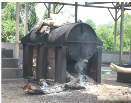
FIGURE 15 Examples of cooking apparatus used to cook animal carcasses to be fed to farmed freshwater fish
