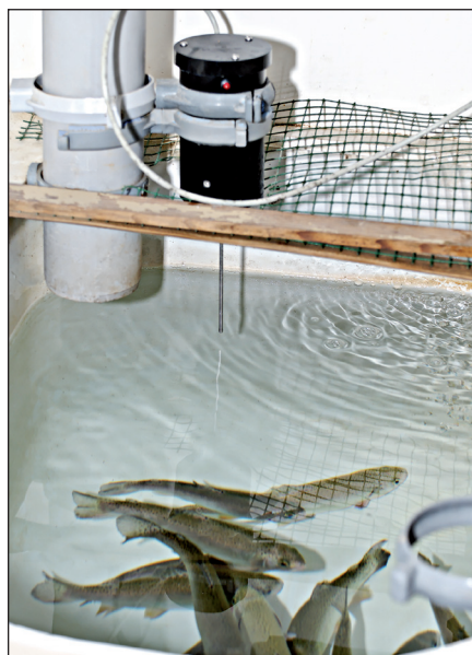
FIGURE 14 Eater-meter device used for experimental studies for monitoring feeding behaviour, feeding rhythms and feed preferences in fish
