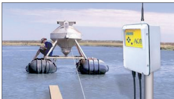
FIGURE 19 Diagram and photo of hydrophone feeding control systems: sensor-based feeding control for pond aquaculture
