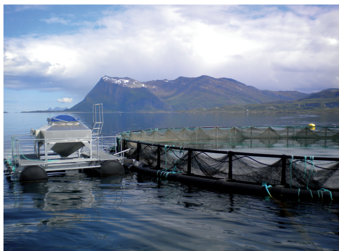
FIGURE 10 Feed distribution using an automatic feeder for cage culture of Atlantic salmon near Bodo in Norway
