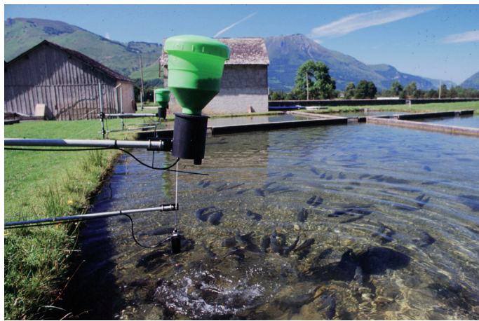
FIGURE 7 A demand feeder used in a rainbow trout farm
