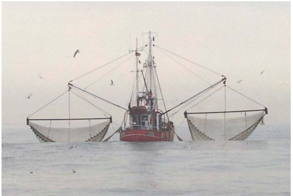
Figure 8: Typical twin-rig shrimp beam trawler.
