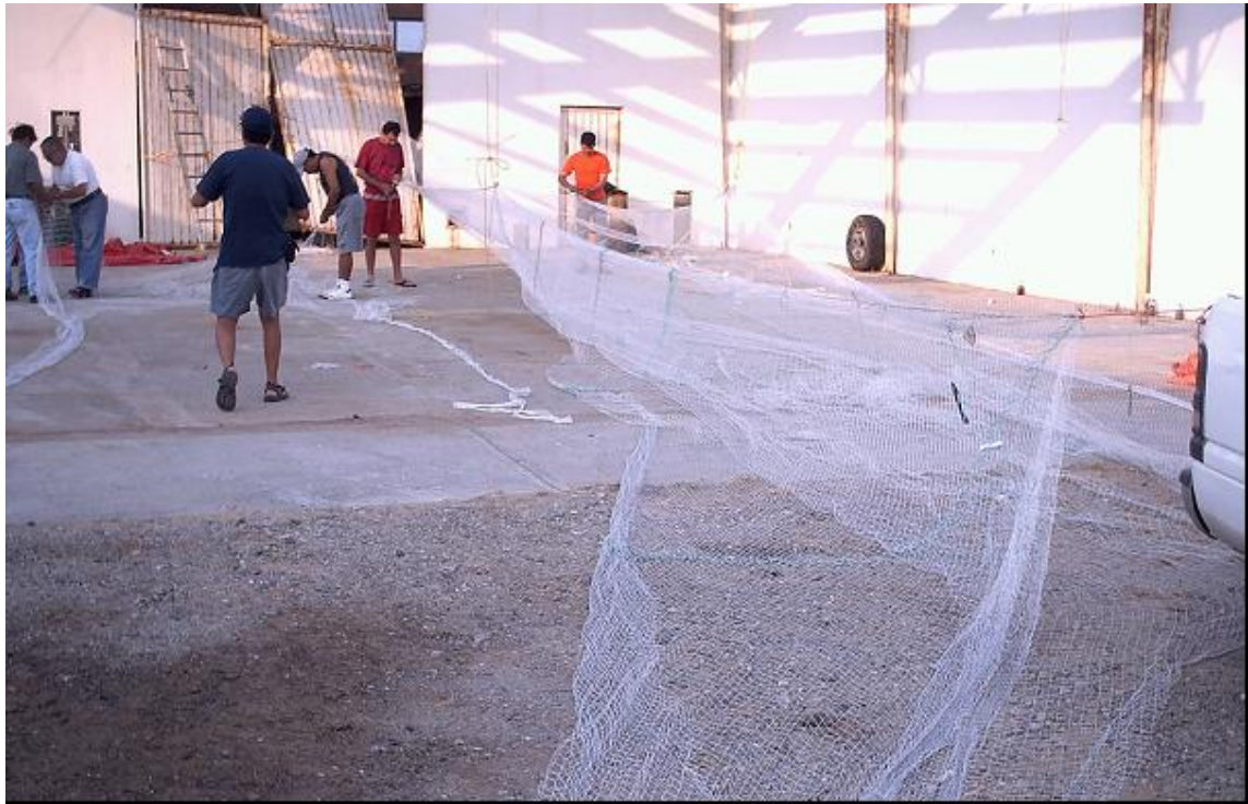
Preparation of side, upper and lower panels for hanging of lateral ropes
