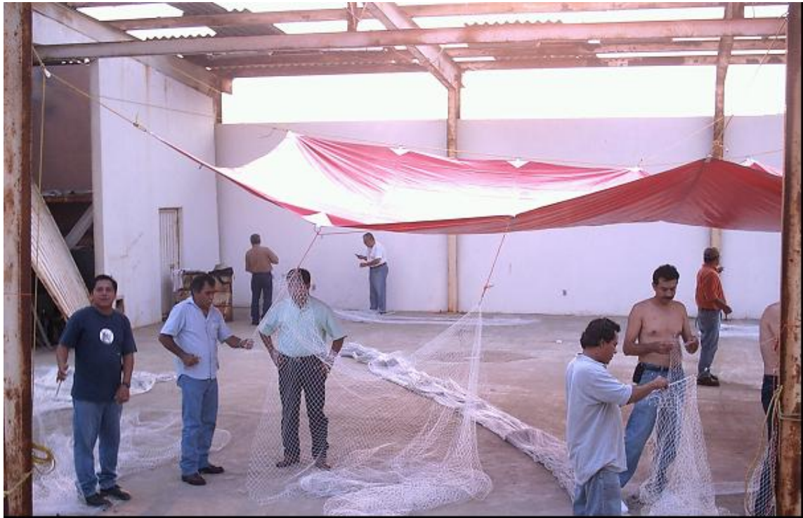
Cutting of netting materials and reinforcing edges
