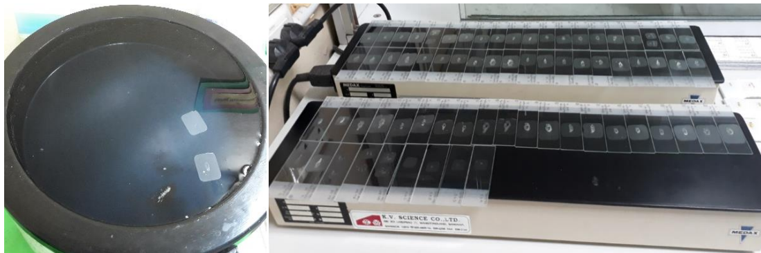
Float the tissue ribbon onto the surface of a \sim 45^\circ\text{C} water bath before placing sections onto slides
