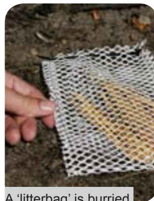
A 'litterbag' is buried in soil to assess litter degradation.
