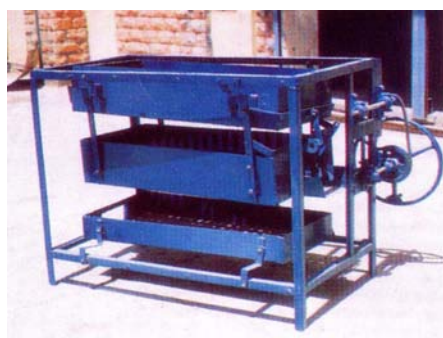
Improved ber grader, developed at CAZRI, Jodhpur, India
