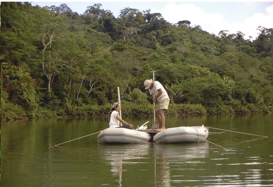
Selection of coring site and anchoring
