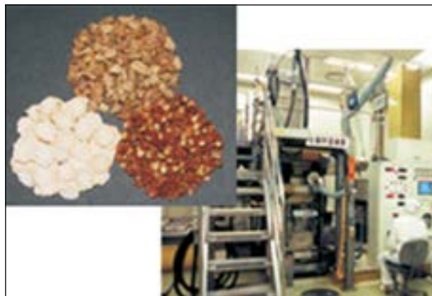
5(b) Crude drugs cut into proper size with cutting machines
