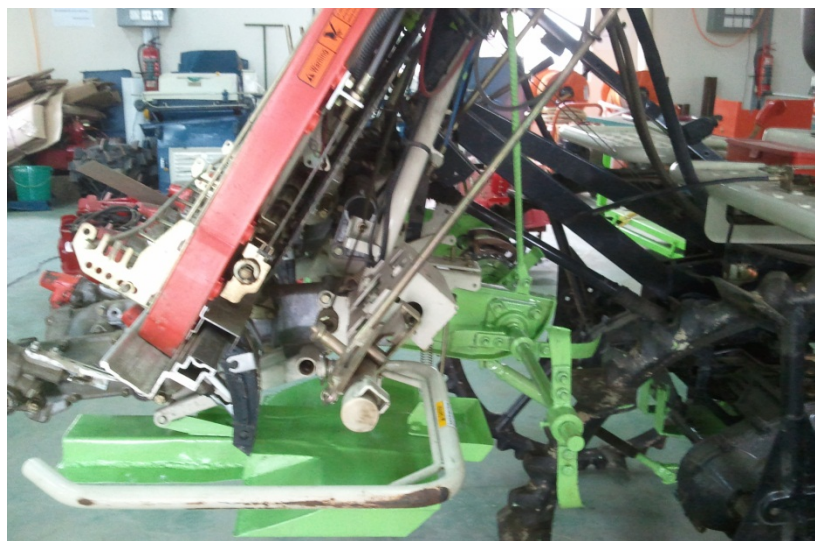
Figure 1. Rice transplanter developed for unpuddled transplanting
