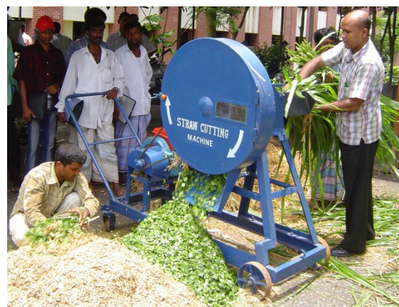
Figure 1. Power Straw and Fodder Chopper (PSFC) being demonstrated.
