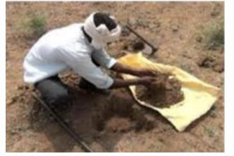
Collect 10 to 100 kg of soils that represent soils you will analyse.
