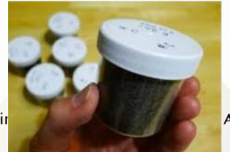
Crush and sieve at 2 mm, store in smaller container (1 or 2 kg).
