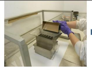
Division into individual parts must be carried out in a way that is representative by reducing the variation between sub-samples
