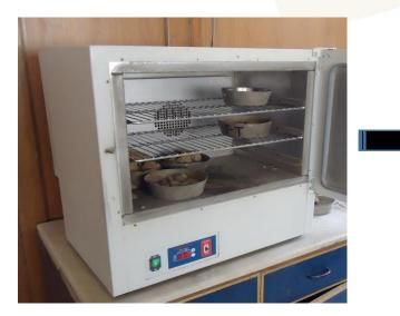
Air drying in a ventilated area or drying Oven at slightly above ambient temperature is preferable  $(35 \pm 5 \ ^{\circ}C)$
