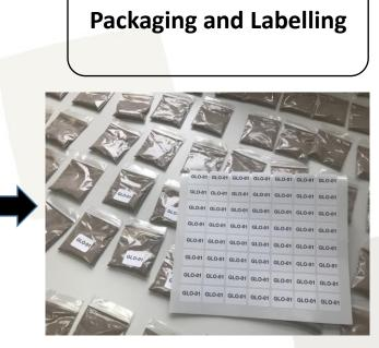
Samples should be placed in bags to protect them from moisture, pests, spillage or contamination
