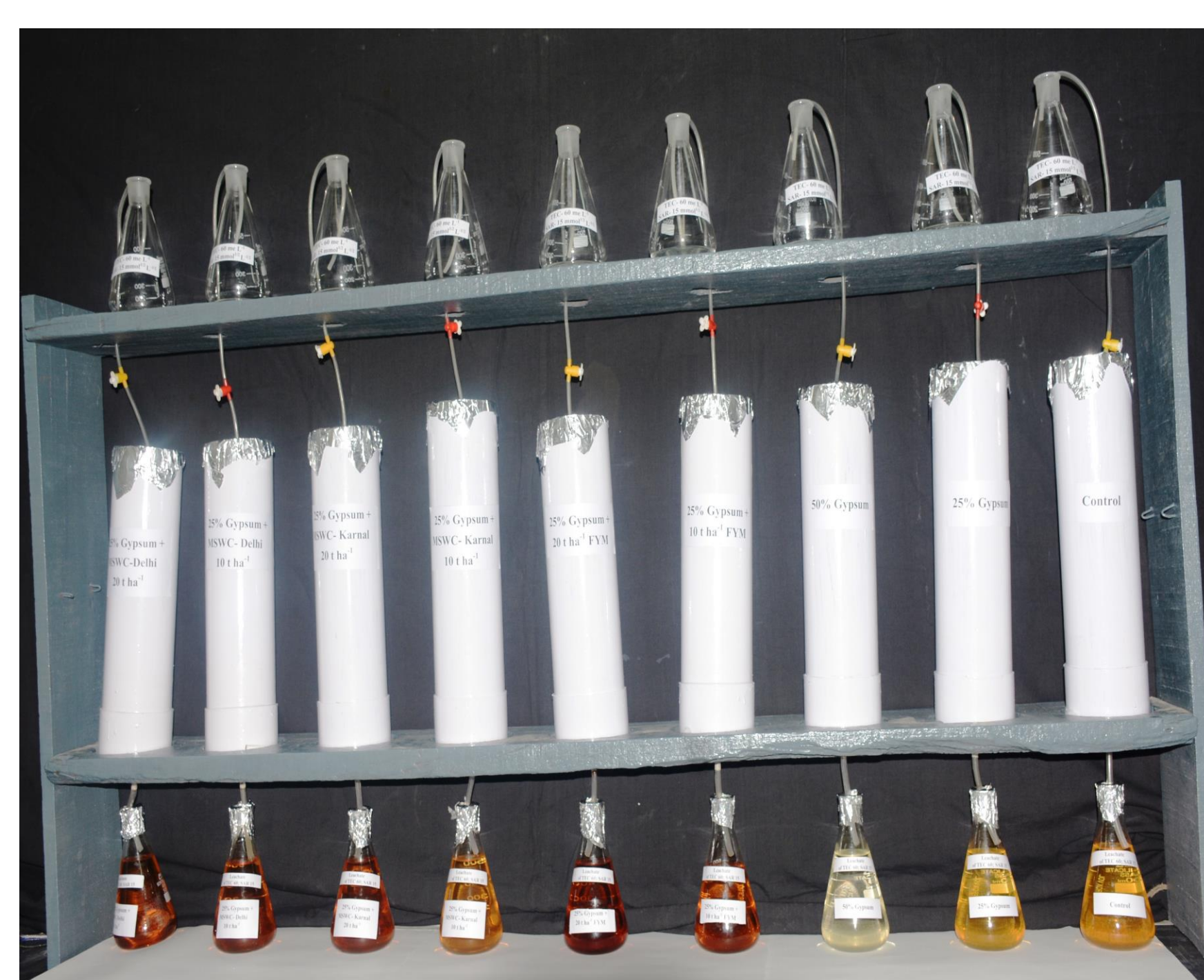
Fig 1. Soil column leaching experiment
