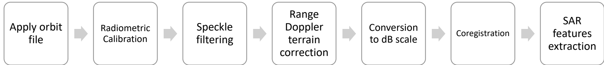
Figure 3: Workflow of radar data processing for ERS-1/2 and Sentinel-1 SAR sensors
