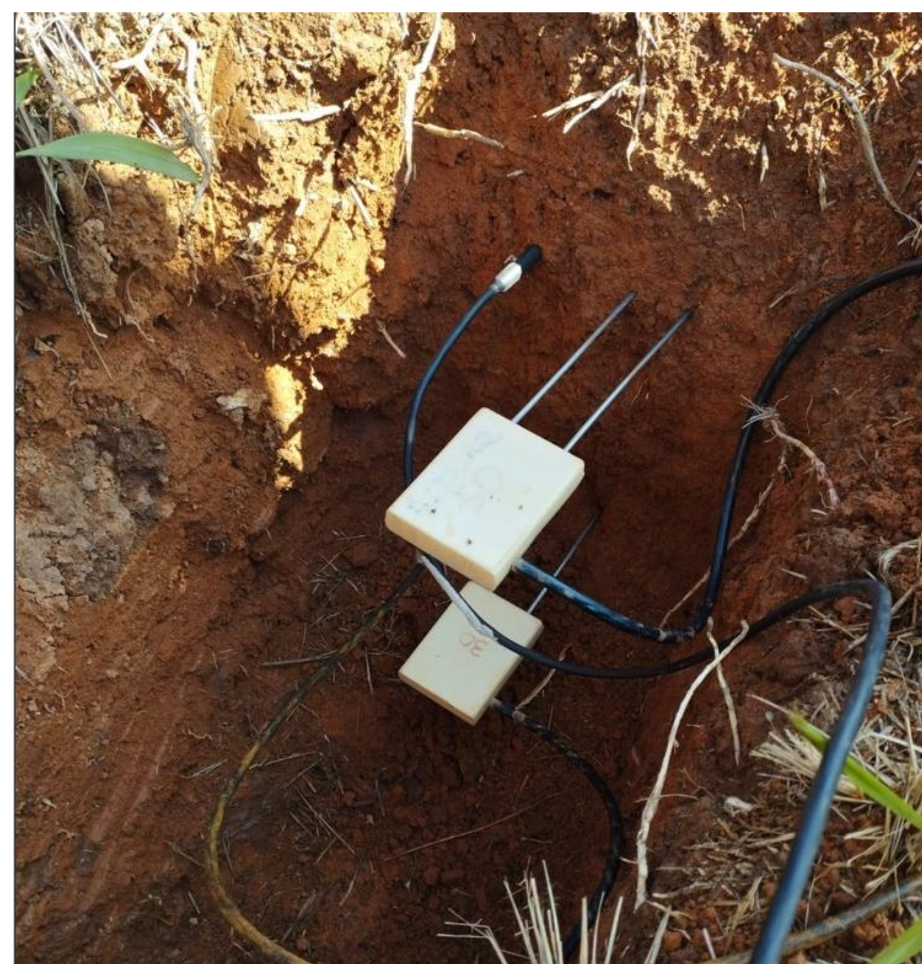
Figure 1. Temperature and humidity sensors installed at 10 and 50 cm in the soil.
