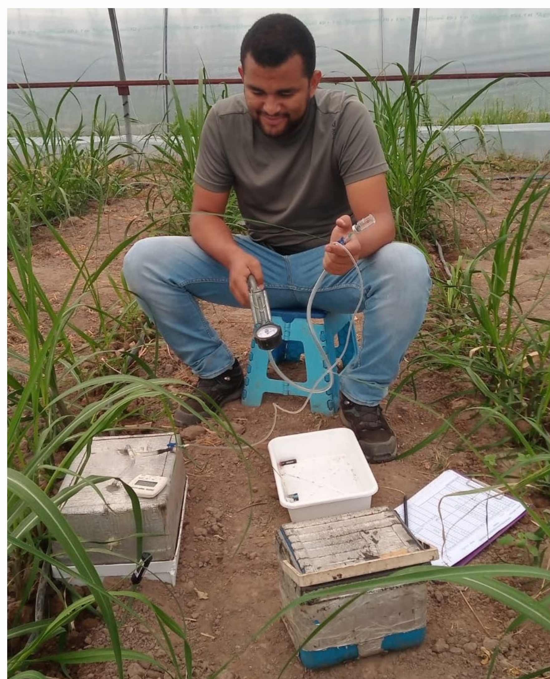
Fig. 2. Gas sampling by static chamber method
