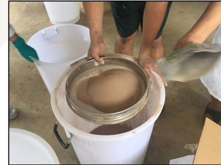
Sieve through 2 mm and then through 0.5 mm
