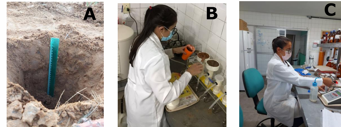
Figure 1: (A) Soil collection in the 30cm profile; (B) Preparation of soil samples in the laboratory; (C) EC analysis
