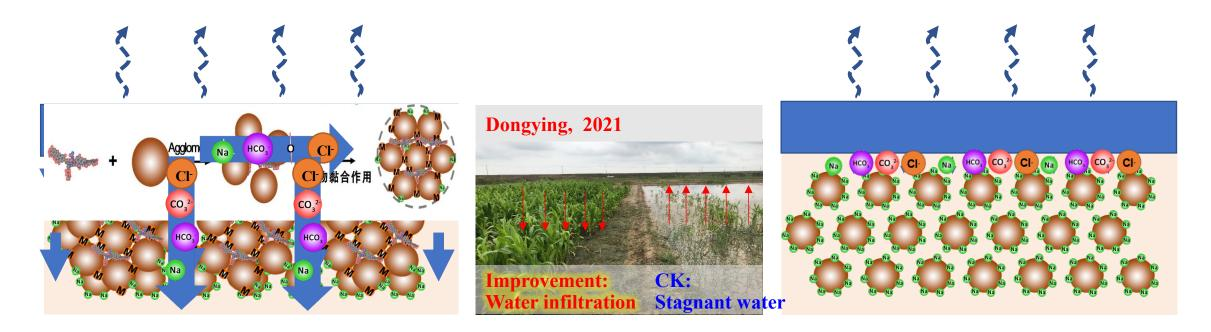
Soil aggregate was formed by the novel amendments, increased soil porosity, and improved the efficiency of salt washing by more than tenfold
